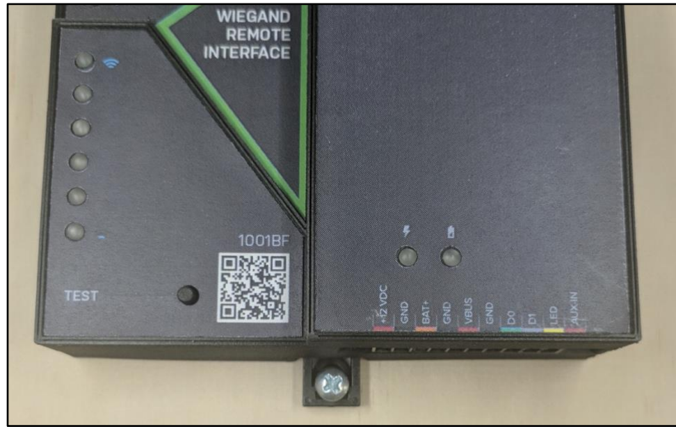
Figure 9: The bottom screw is shown mounted through the black DIN clip to the wall:
