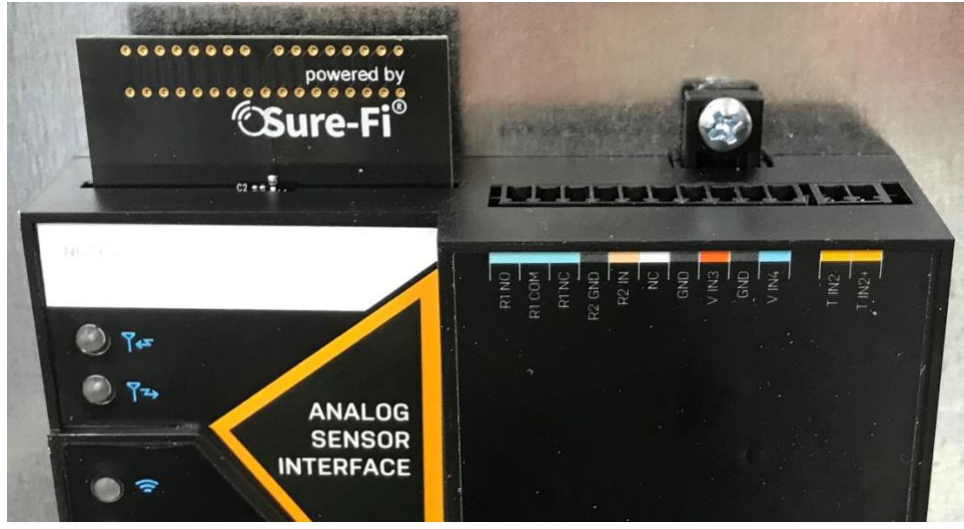
Figure 4: The top screw is shown mounted through the DIN clip to the wall:
