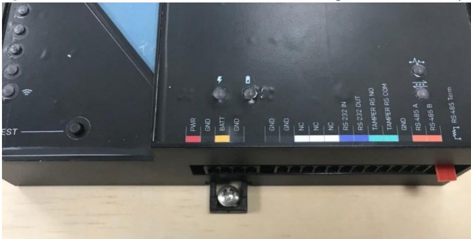
Figure 9: The bottom screw is shown mounted through the black DIN clip to the wall:
